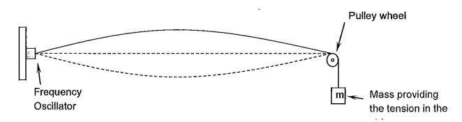
Using this apparatus the mass providing the tension in the string was altered over several trials; each trial the frequency was varied until resonance occurred and produced the fundamental standing wave pictured above. The results are shown in the table below.
